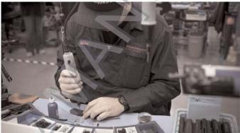
Every Benchmade knife is assembled by hand, and it's no surprise that there are more hand operations performed at this point in a knife's production than at any other stage in the process. An assembly technician receives all of the components — blade, liner, handle, hardware — and carefully pieces them together. The technician checks the knife for blade play (movement from side-to-side and up-and-down), and the result is a knife just waiting to be sharpened.
