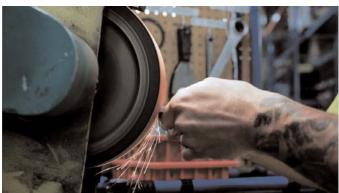
It takes longer to master blade sharpening than any other skill. A sharpening technician puts a razor edge on the knife using a standing belt sander, and this step takes extraordinary concentration. Each blade is sharpened to a targeted 30-degree inclusive angle, 15 degrees on each side. The knife is sharp enough when it can cut through ultra-thin phonebook paper effortlessly without tearing. And only then is it truly a Benchmade.
