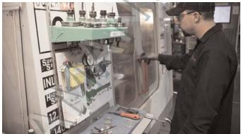
Blade holes, handles and grooves are cut-on high-speed mills. For every job (or batch), the blade milling technician programs the mill and measures the blade or handle to make sure it meets our precise tolerances. Blades and handles differ from knife to knife, so the technician gathers a specific set of measuring tools for each job.
